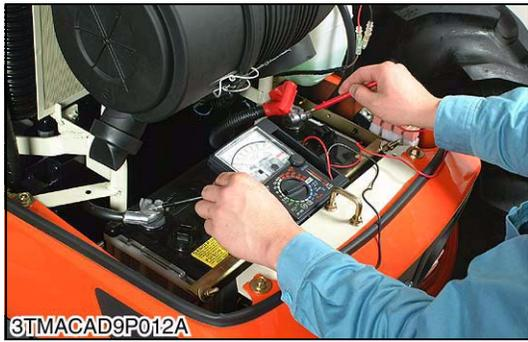
**Alternator on Unit Test
