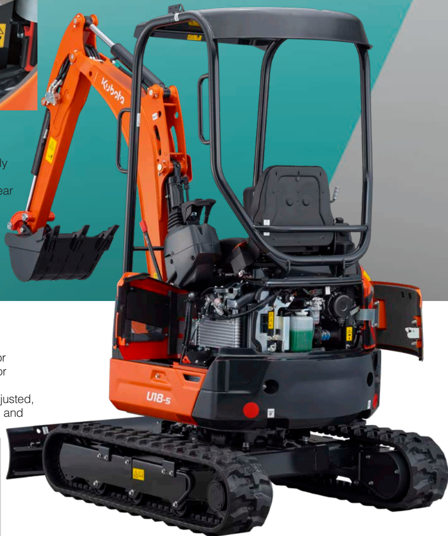
A. Air cleaner C. Starter motor B. Water separator D. Oil dipstick
